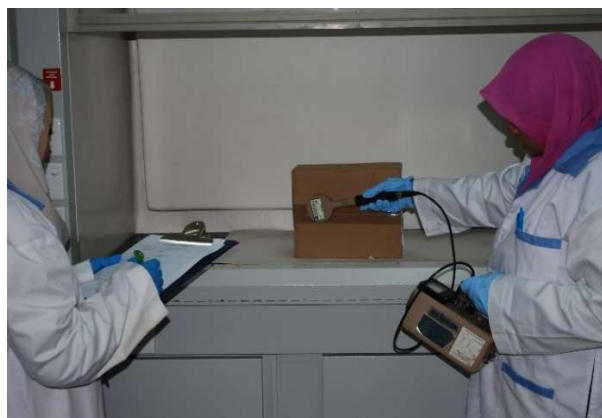
Figure 2. Radiation detection instruments are used to assess external dose rates and surface contamination before samples are opened or processed.
