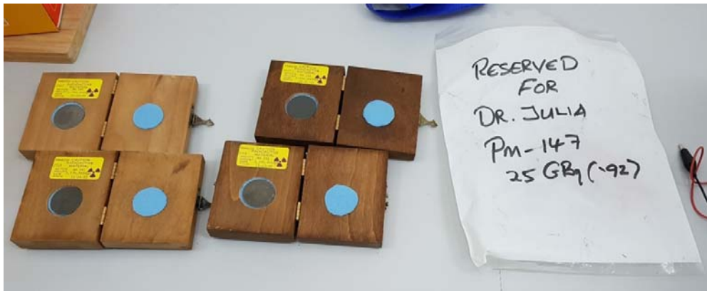
From left to right: Am-241 samples (stored in wooden container together with black metallic disks) and a package of Pm-147.
