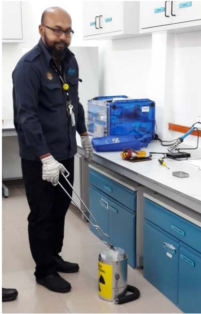
The sample was taking out from a shielded canister (left) and then was weight using a balance (right).
