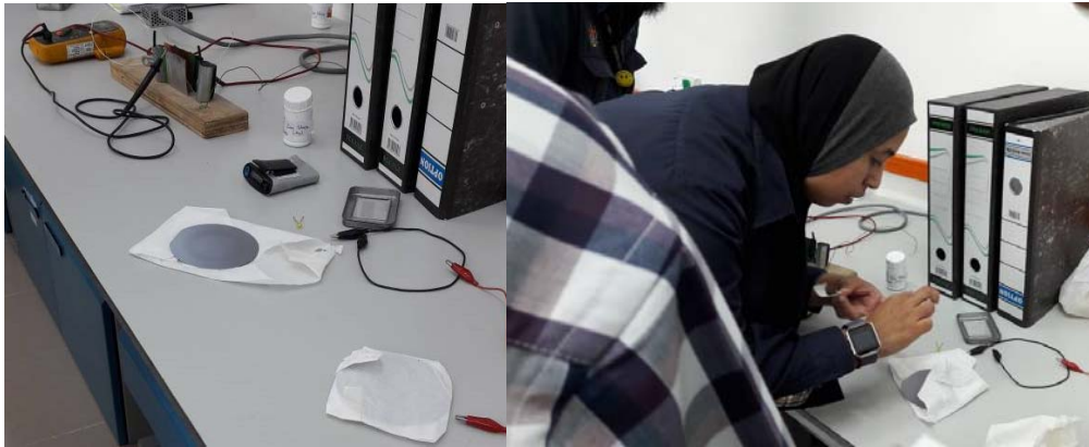
Setting up the silicon electrode betavoltaic cell.
