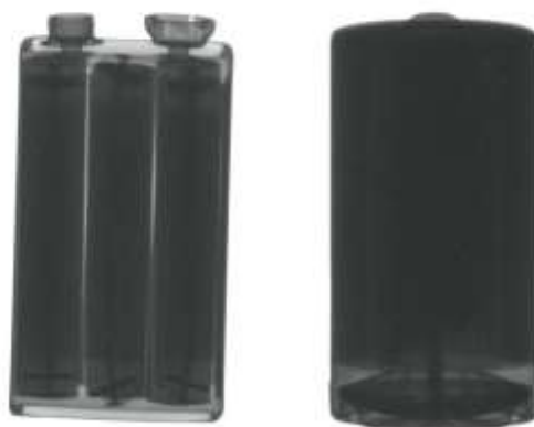
Figure 8. X-ray radiography of internal structure of Lithium battery using new advance detector with X-ray scintillator
