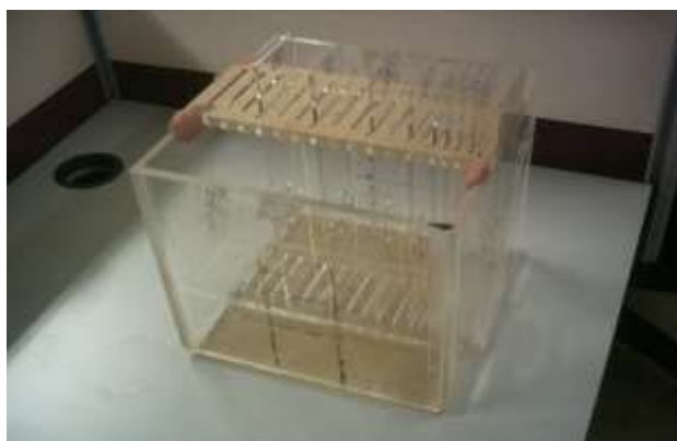
Figure 2. Water Phantom used in this research
