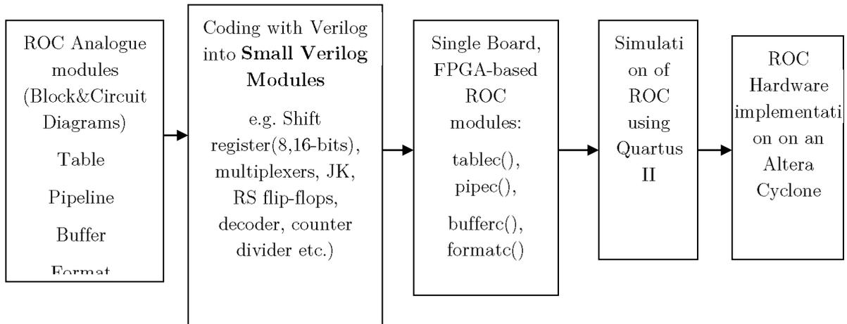
Figure 2. The analogue modules of readout control (ROC) of the ZEUS detector were coded into single board, FPGA-based using Verilog, starting with basic blocks, later combined to become the main controlling block before being simulated on Quartus II.
