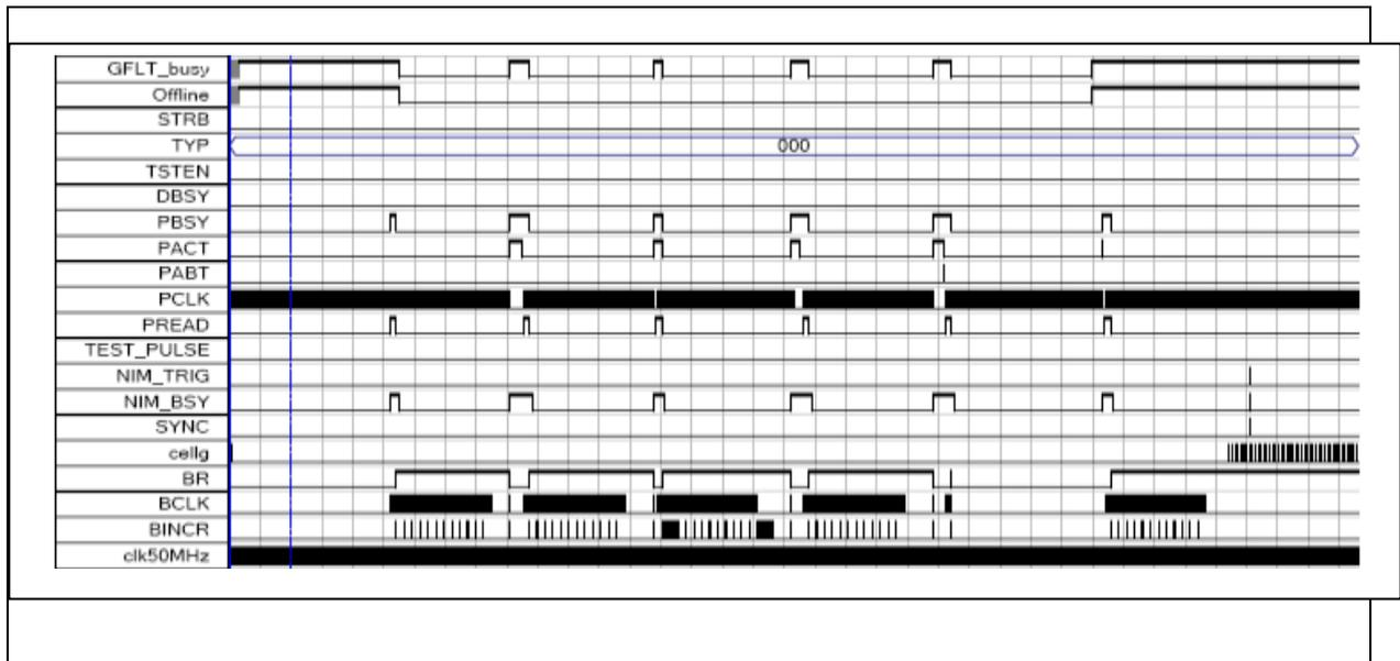
Figure 6a. Output signals from the FPGA-based readout control
