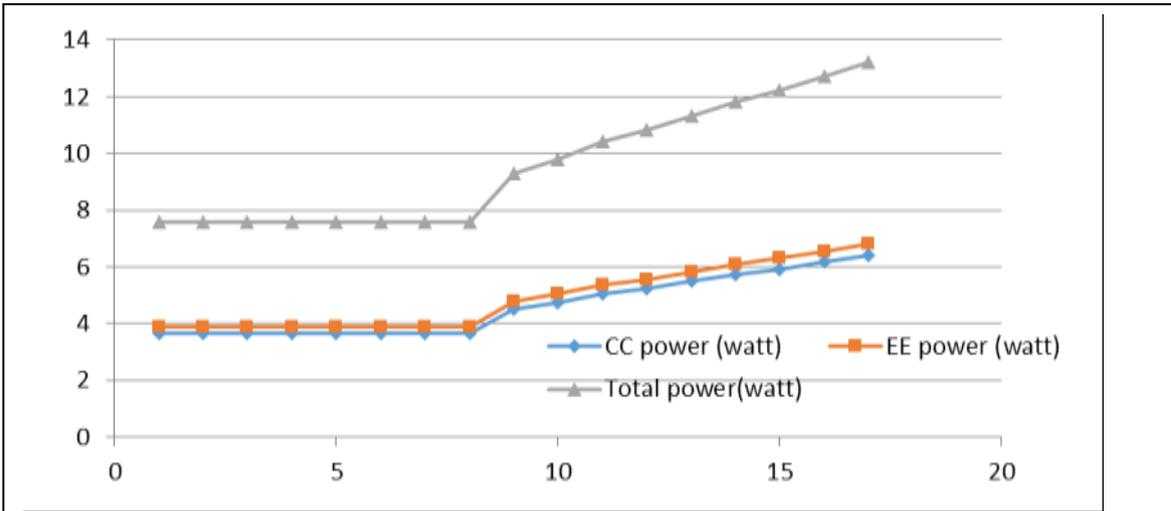
Figure 10. Plot of power (watt) from bias drain and emitter current and their total power versus number of chips of quad TTL-ECL quad translator type (MC0124)
