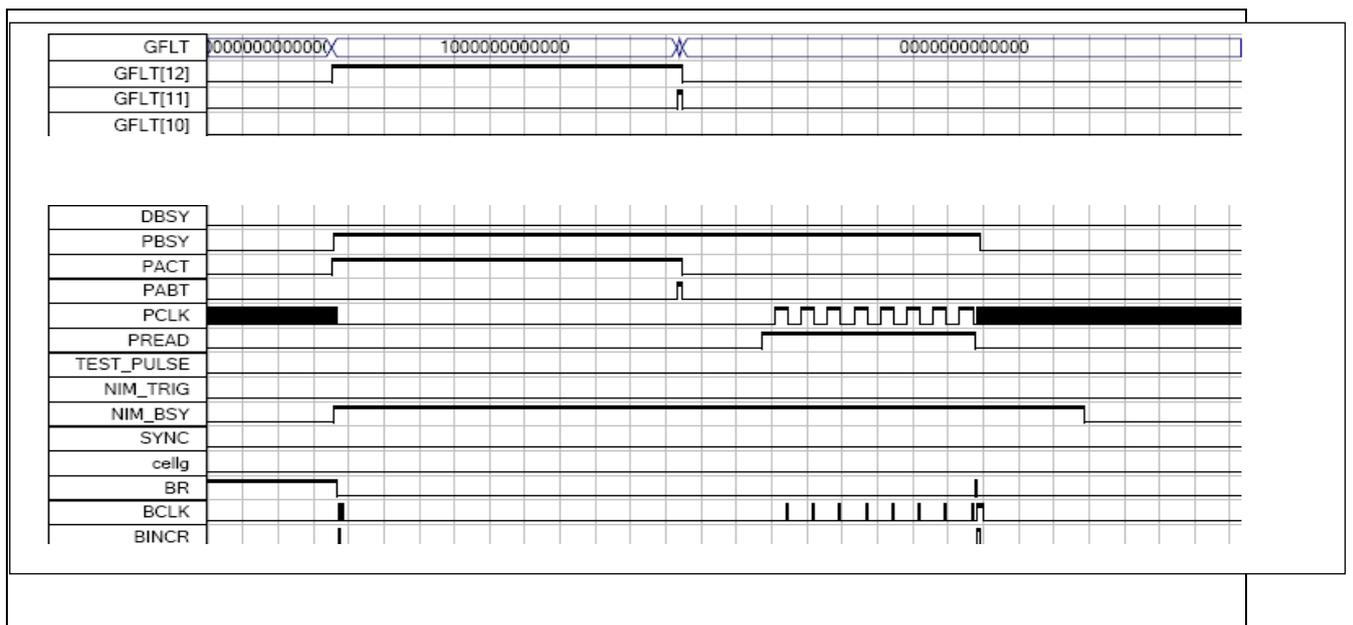
Figure 6b. A close-up of the FPGA-based readout control showing the abort ABT signal from the pipeline control. Global first level trigger during on-line operation with GFLT[12]: ACT=1 for Accept data trigger, while GFLT[11]: ABT=1 for Abort data trigger (CP: HERA clock 10MHz).
