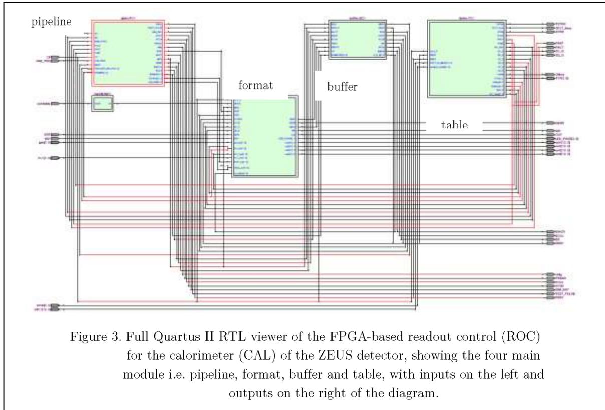
Figure 3. Full Quartus II RTL viewer of the FPGA-based readout control (ROC) for the calorimeter (CAL) of the ZEUS detector, showing the four main module i.e. pipeline, format, buffer and table, with inputs on the left and outputs on the right of the diagram.
