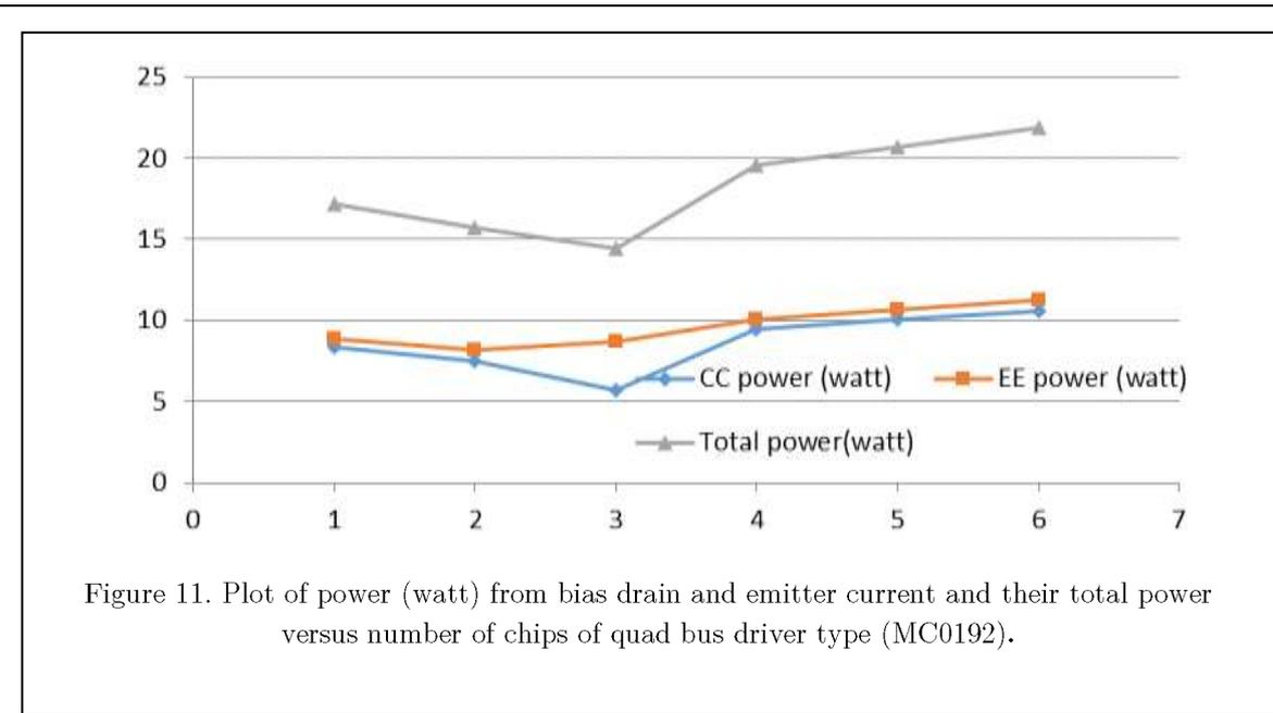
Figure 11. Plot of power (watt) from bias drain and emitter current and their total power versus number of chips of quad bus driver type (MC0192).
