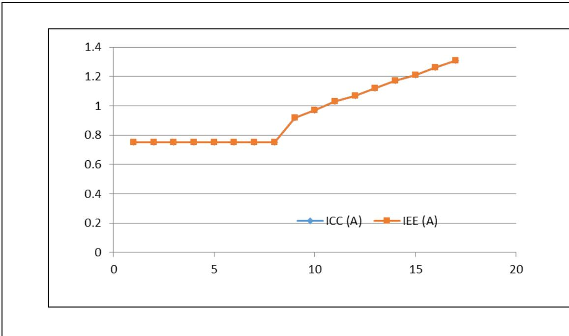
Figure 8. Plot of current  $I_{CC}$  (A) and  $I_{EE}$  (A) versus number of chips of TTL-ECL quad translator type (MC0124) showing the tendency the currents to increase with the number of chips
