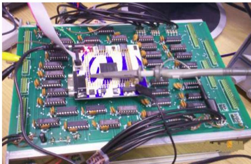
Figure 7. A 7inch by 11inch (17.5cm by 27.5cm) PCB designed using Proteus software, with the FPGA Altera Cyclone mounted in the middle and TTL-ECL, ECL-TTL and Quad Bus Driver chips mounted fully. The PCB was tested in laboratory using frequency generator and high current voltage supply
