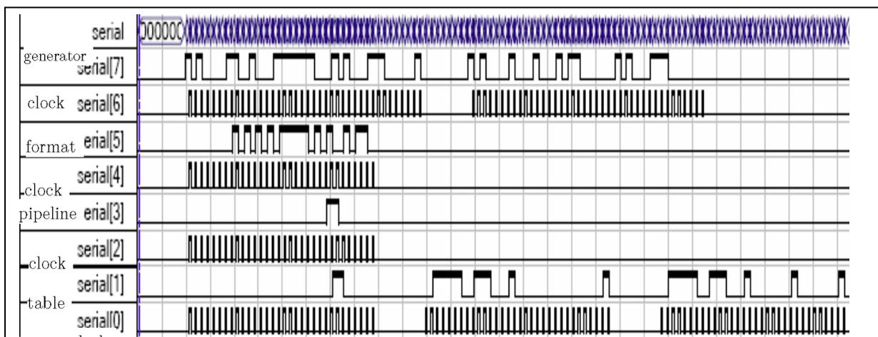
Figure 5. Serial data input to the FPGA-based readout control during off-line mode (serial[0] for table control, serial[3] for pipeline, serial[5] for format control, serial[7] for generator control; while serial[0],[2],[4],[6] were serial clock 10MHz)
