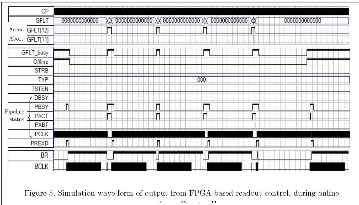
Figure 5. Simulation wave form of output from FPGA-based readout control, during online
