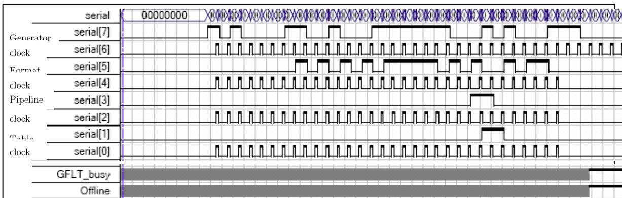
Figure 4. Simulation wave form of 16-bits serial input data for readout control, during offline, with negative edge clock trigger on Quartus II
